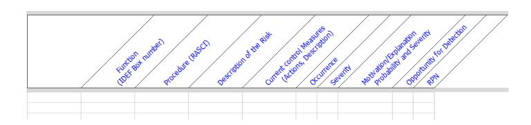
**Figure 2.** Typical header fields for a FMEA risk analysis. For the first column, Function (or Process), the IDEFO box number suffices. The field Motivation/Explanation Probability and Severity isn't mandatory, but it can help to record key points and to reach similar conclusions at a later point in time. RPN = Occurrence x Severity x Detection
